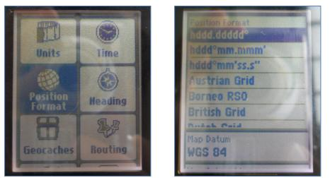
7. Scroll down to the MAP DATUM and MAP SPHEROID options. The default options for both categories should be WGS 84. If this is the case, LEAVE THE OPTIONS as is. If not, press in on the knob over each option respectively and press the KNOB DOWN to scroll to select WGS 84.
