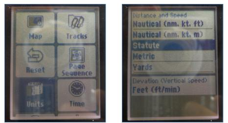
3. Press the KNOB DOWN to the ELEVATION drop down menu and press in on the knob to select it. Scroll to Meters if you selected Metric in the Distance and Speed menu above or Feet (ft/min) if you previously selected Statue. Press in on the knob to make your selection.
